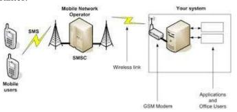
Gambar 2. Diagram kerja SMS Gateway
